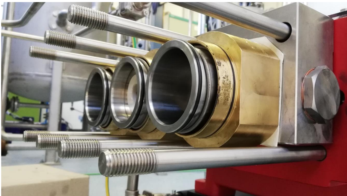
Figure 7 : View into the open piston chamber of the triplex pump
