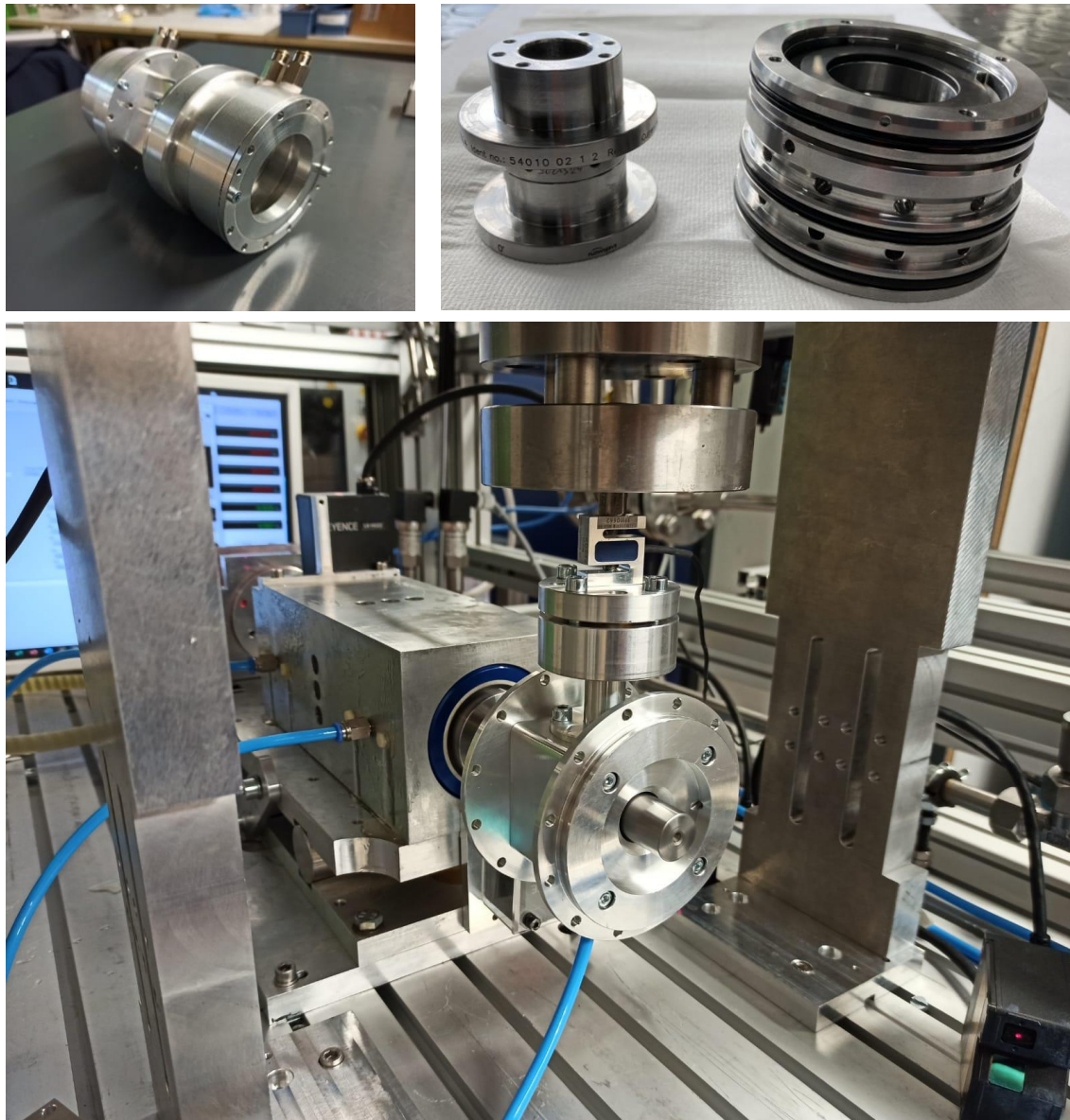
Figure 8: Aerostatic gas bearing - bearing housing (top left), seals (top right) and test rig during initial air commissioning tests (bottom)
