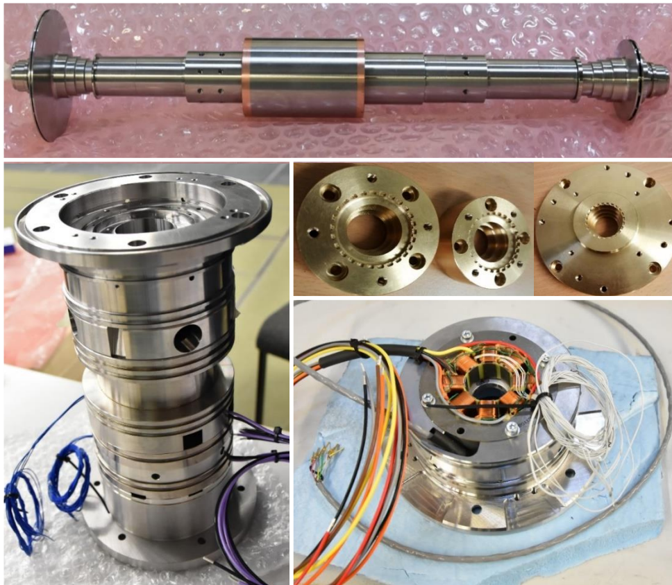
Figure 11: Parts of the turbomachine – rotor with assembled impellers and generator without bearing parts (top), Labyrinth seals (middle), test assembly of internal stator parts (bottom left), assembled radial bearing (bottom right)
